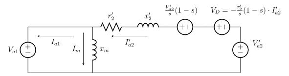
**Figure 2:** The generator circuit from Figure 1 with the developed power  $P_d$  pieces separated from the constant values for  $V'_{a2}$  and  $x'_2$ .
