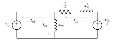
**Figure 1:** The generator circuit representation showing the lack of the stator impedance.
